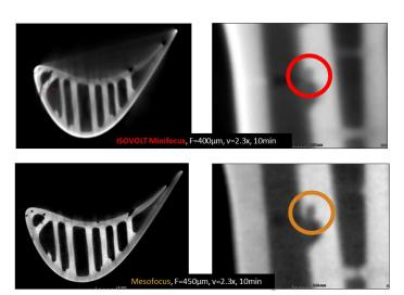
The results of Mini- versus Mesofocus in the example of blade inspection.
